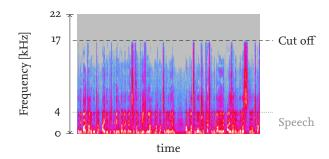
Figure 9: Spectrogram of DVB-T recording. Note that audio frequencies above 17 kHz are cut off.
