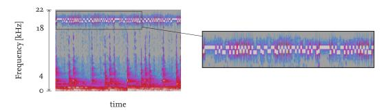
Figure 7: Spectrogram of a disclosed Lisnr audio beacon. An FSK scheme encodes a repeating bit sequence in the near-ultrasonic frequency range between 18.5 and 19.5 kHz.
