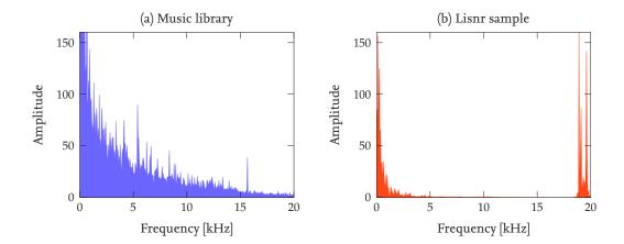
Figure 4: Plot (a) shows the frequency distribution of more than 1,500 songs whereas Figure (b) depicts the frequency distribution of an audio sample containing a Lisnr audio beacon.
