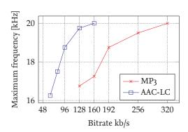
Figure 10: Frequency bandwidth of MP3 and AAC.
