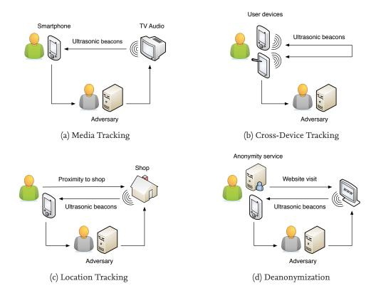
Figure 1: Examples of different privacy threats introduced by ultrasonic side channels. (a) Ultrasonic beacons are embedded in TV audio to track the viewing habits of a user; (b) ultrasonic beacons are used to track a user across multiple devices; (c) the user's location is precisely tracked inside a store using ultrasonic signals; (d) visitors of a website are de-anonymized through ultrasonic beacons sent by the website.
