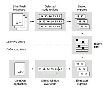
Figure 5: Schematic depiction of the detection method for mobile applications that employ inaudible sound.
