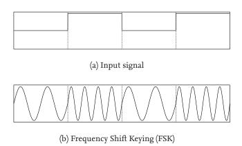
Figure 3: Information encoding using FSK modulation.
