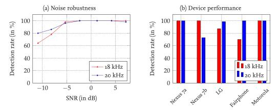
Figure 8: Results for the device experiment. Figure (a) presents the detection performance vs. signal-to-noise ratio for different frequency bands and (b) the detection performance for different frequency bands and mobile devices.
