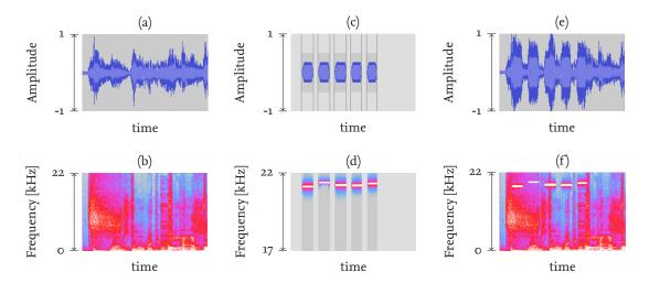
Figure 6: Example of transmission of ultrasonic beacons. The upper three panels depict the audio wave of an audio signal, while the lower three panels show the corresponding Spectrogram. (a)-(b) show a music track, (c)-(d) a ultrasonic beacon, (e)-(f) shows the result after embedding the beacon into the original track.
